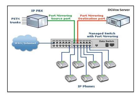
As shown in the diagram above, the port mirroring can be done on a managed switch and the destination port should be connected to the LAN card in the DGVox application server.
